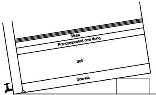
Figure 1: Illustration of Vermicomposting Leachate Reactor.
