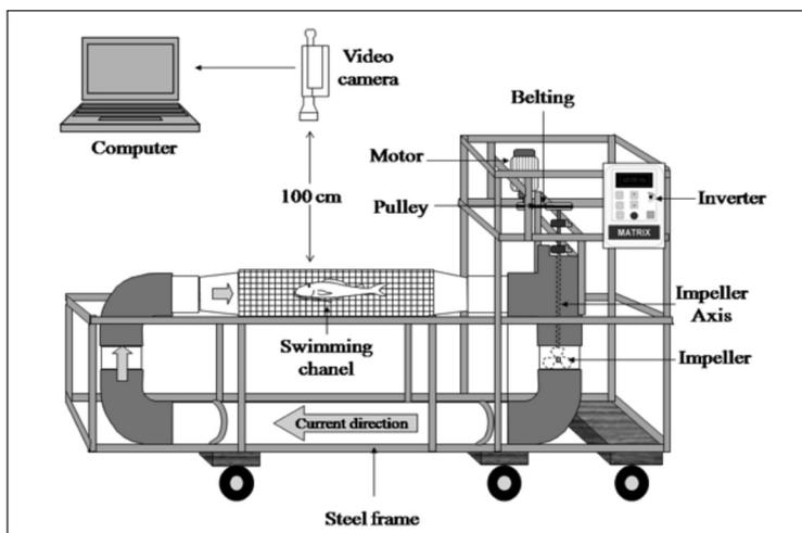
Figure 1: Schematic observation of fish behavior for swimming speed and endurance for asian redbtail catfish (*Hemibagrus nemurus*) by PVC-made flume tank
