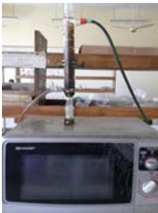
Figure 2: Modified domestic microwave assisted transesterification
