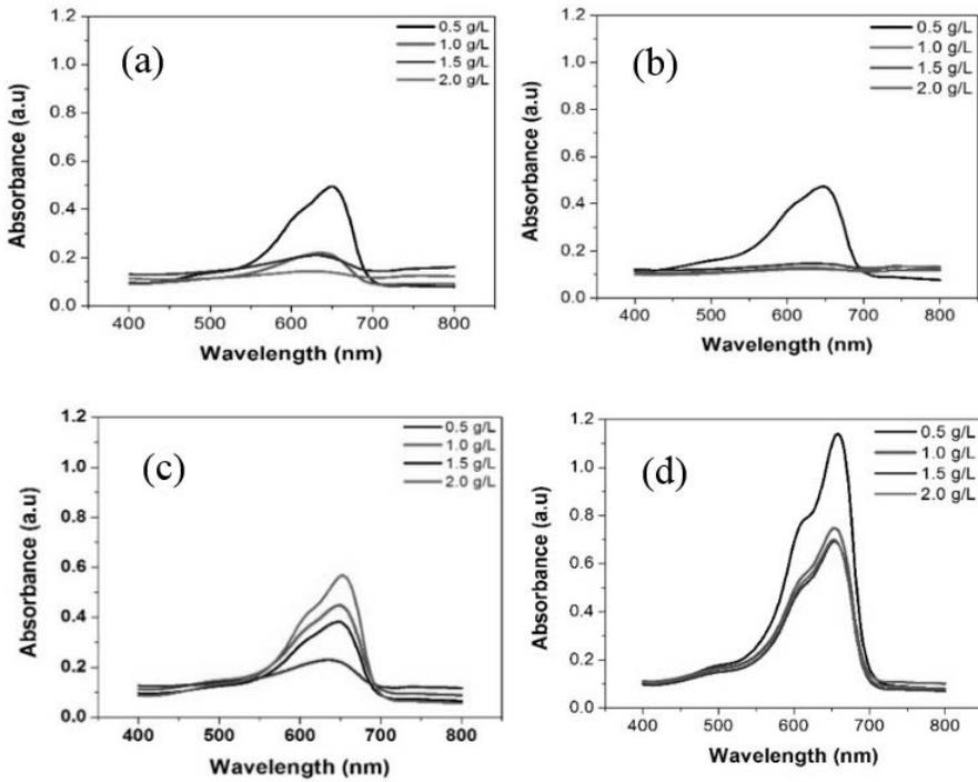
Figure 4: UV Vis spectra of MB dye solution after treatment with a) 1 mol % Er doped ZnO (b) 1 mol % Ce doped ZnO (c) 1 mol % La doped ZnO and (d) 1 mol % Pr doped ZnO photocatalysts
