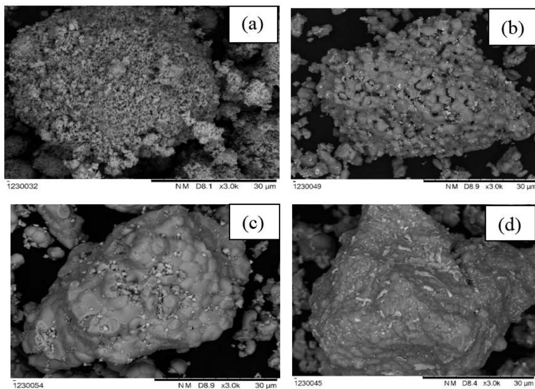
Figure 2: Backscattered electron images of 1 mol % (a) Er doped ZnO, (b) Ce doped ZnO, (c) La doped ZnO and (d) Pr doped ZnO.
