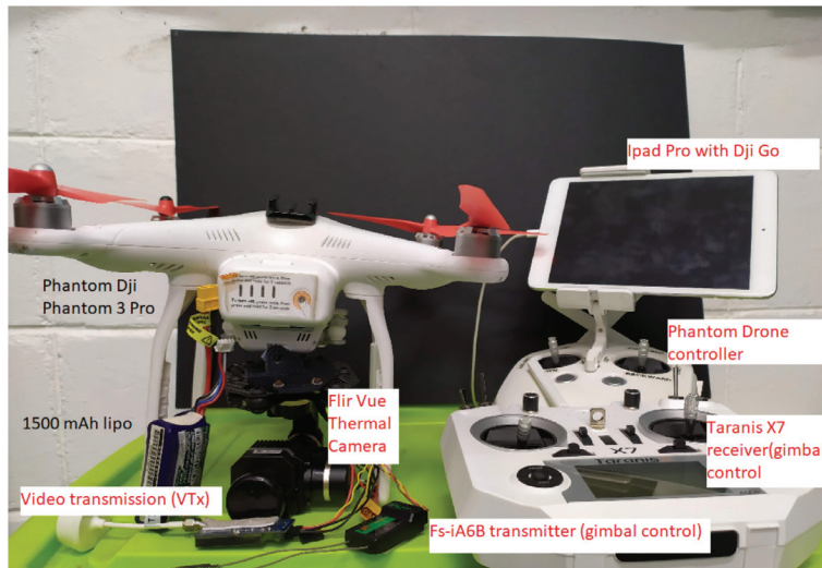
Figure 2: Setup of the thermal camera equipped drone
