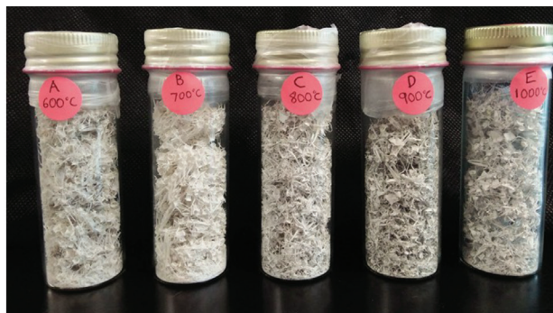
Figure 4: Comparison of the colour of spotted sardinella bone heated at different temperatures
