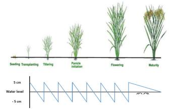
Figure 2: Schematic diagrams of water level control for field irrigation in AWD method
