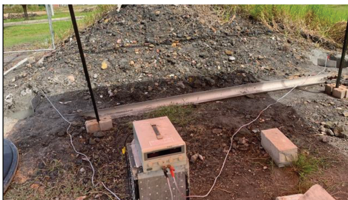
Figure 6: In situ electrokinetic remediation (EKR) set up using cementation method as electrolyte compartment
