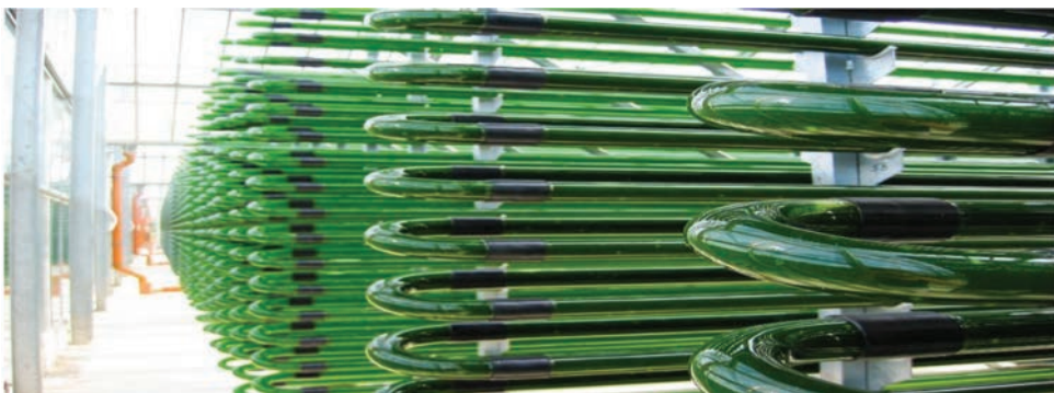
Figure 3: Closed ponds system of microalgae cultivation Sources: www.superfoodevolution.com
