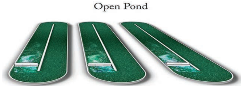
Figure 2: The open-pond system of microalgae cultivation Sources: making-biodiesel-books.com
