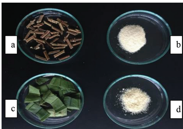
Figure 2: Extraction of cellulose: (a) M. malabathricum branches before treatment, (b) branch cellulose obtained after treatment, (c) M. malabathricum leaves before treatment and (d) leaf cellulose obtained after treatment
