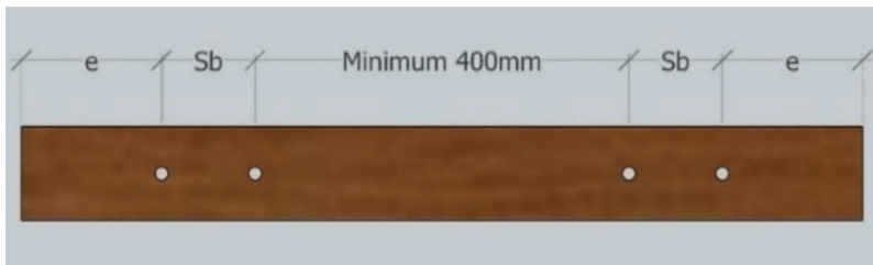
Figure 4: Illustration of bolted-connection configurations
