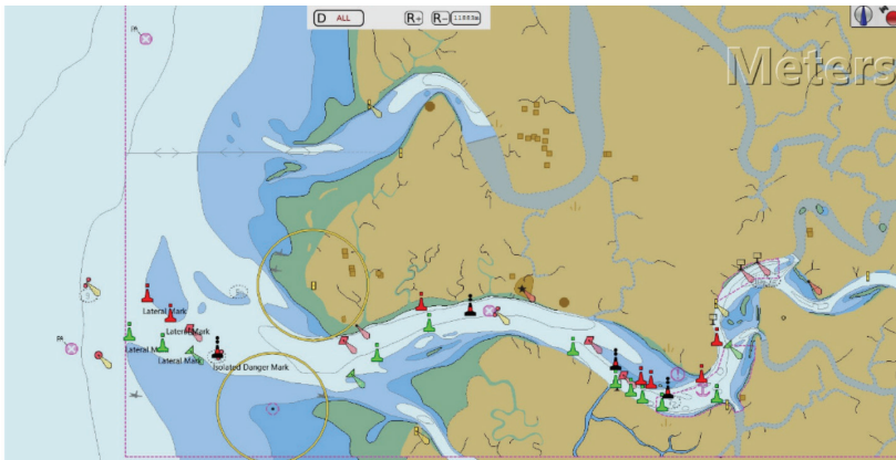
Figure 8: Placement of new navigational aids in Rajang River
