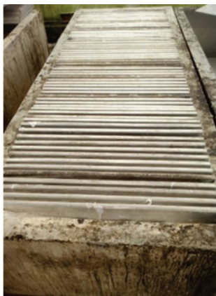
Figure 6: Coagulated latex scraps with Co-act L to produce rubber sheets
