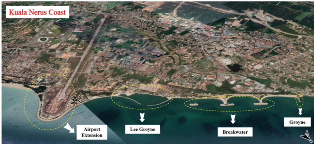
Figure 4: The type of coastal defence in a mitigation plan by DID and the state government with the selected coastal segments' aerial views
