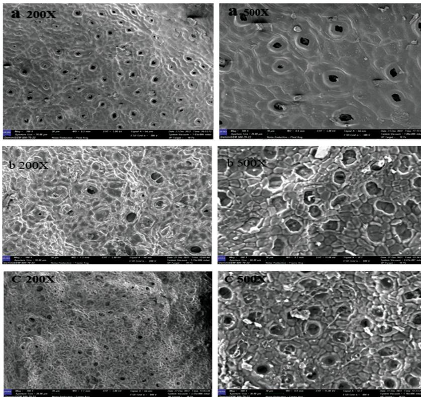
Figure 2: FESEM images of (a) MC-AC1, (b) MC-AC2, and (c) MC-AC3 at 200X and 500X magnification
