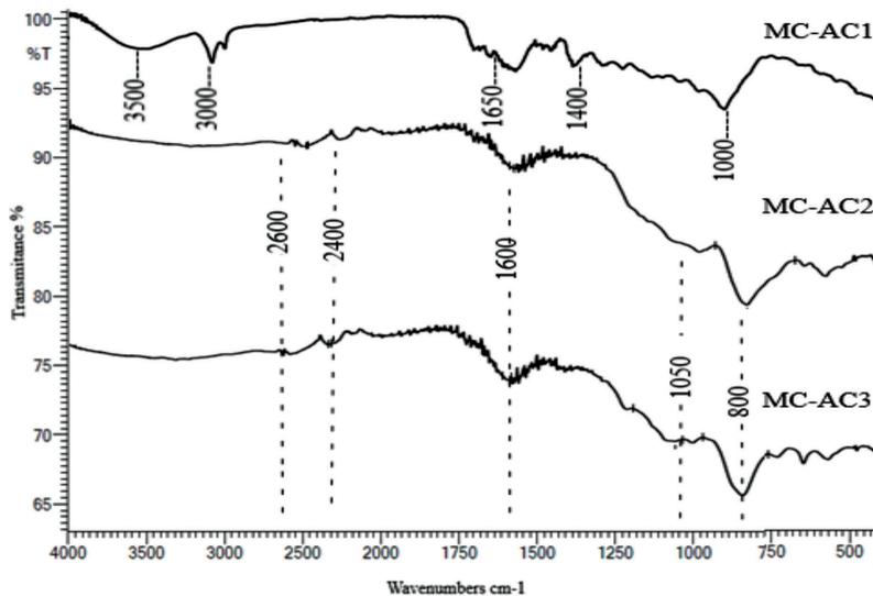
Figure 3: FTIR spectra of the three activated carbons
