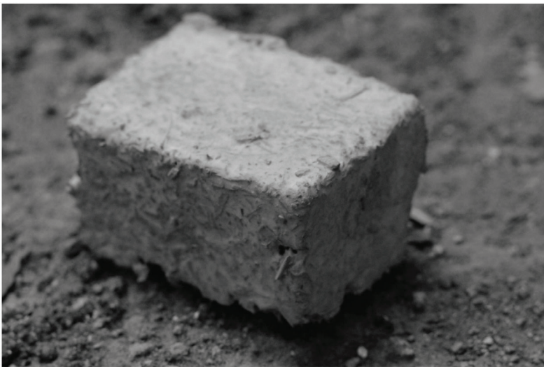
Figure 2: Sample of Pleurotus ostreatus mycelium fully colonised with sawdust substrate and shaped itself according to the container mould
