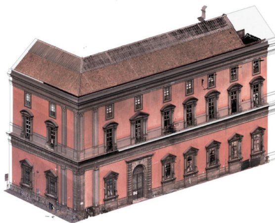
Figure 4: Point cloud superimposed on the HBIM model of the National Archaeological Museum of Naples Source: Martinelli et al. (2022)
