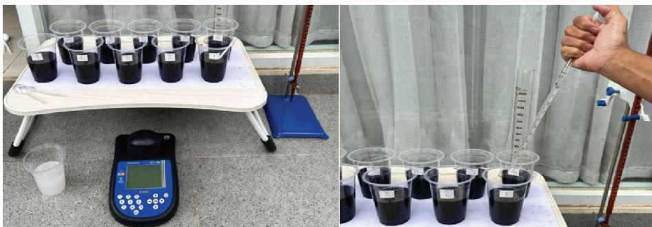
Figure 1: Addition of alum solution to Sasirangan wastewater
