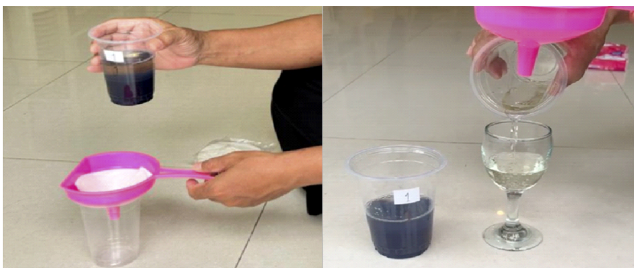
Figure 2: Water filtration to remove light flocs
