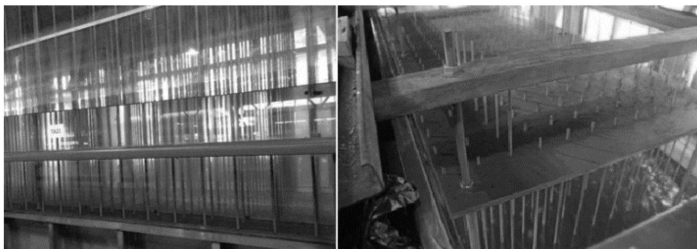
Figure 4: Photos of model with mangrove seedling trees in wave flume
