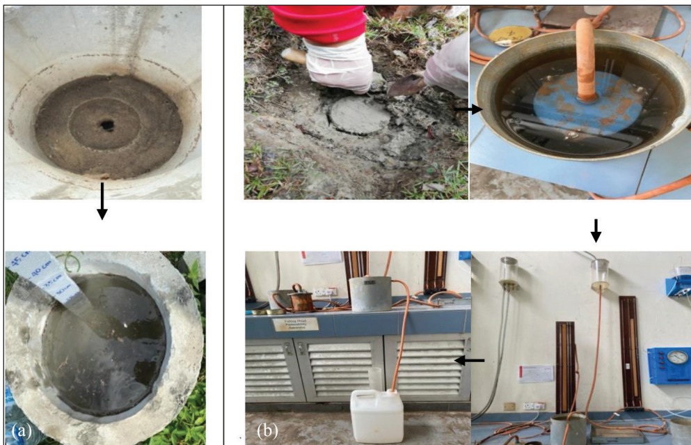
Figure 4: Infiltration rate test, (a) field experiment and (b) falling head laboratory experiment
