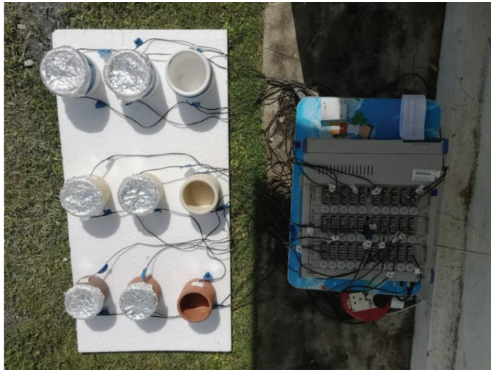
Figure 3: Thermocouples connected to all pots during the experiment
